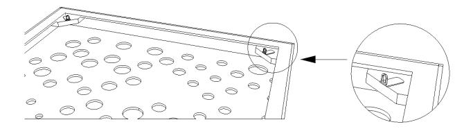
2. Torsion Springs and Tbar connectors for suspension on 15/16 T-bar ceiling grids. Torsion springs and T-bar connectors provided by Sectis. 15/16" T-bar grid to be part of the installation scope.
